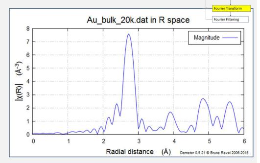
Peak positions (phase shift corrected) => neighbour shells Peak amplitude and shape => number and type of neigbours pre-edge subtraction
