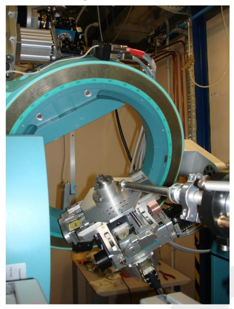
The same diffraction peak is measured for different orientatons of the sample
