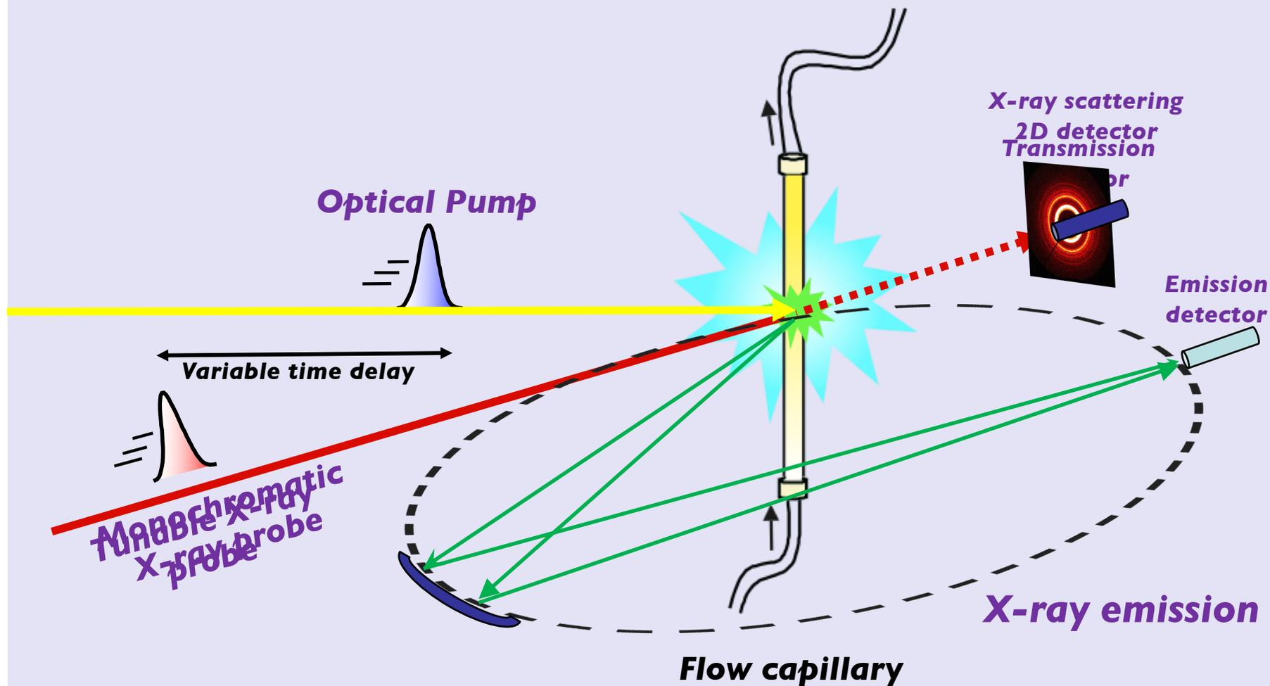
Measured signal= pumped minus unpumped signals
