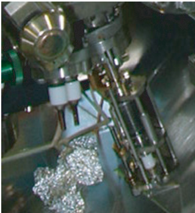
Figure 3.24: Photo of TriCon source mounted on the IPES preparation chamber.
