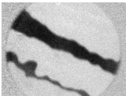
Figure. MCD-PEEM image on Cs/Ni(12 ML)/Cu(001). The excitation source is second harmonics (3.1 eV) of Ti:Sapphire laser. The two domains correspond to up and down magnetization domains.
