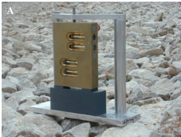
Fig. 3: (A) Photography of the sample holder block. (B) Sketch of the Block: Up to four samples can be thermostated at the same time.
