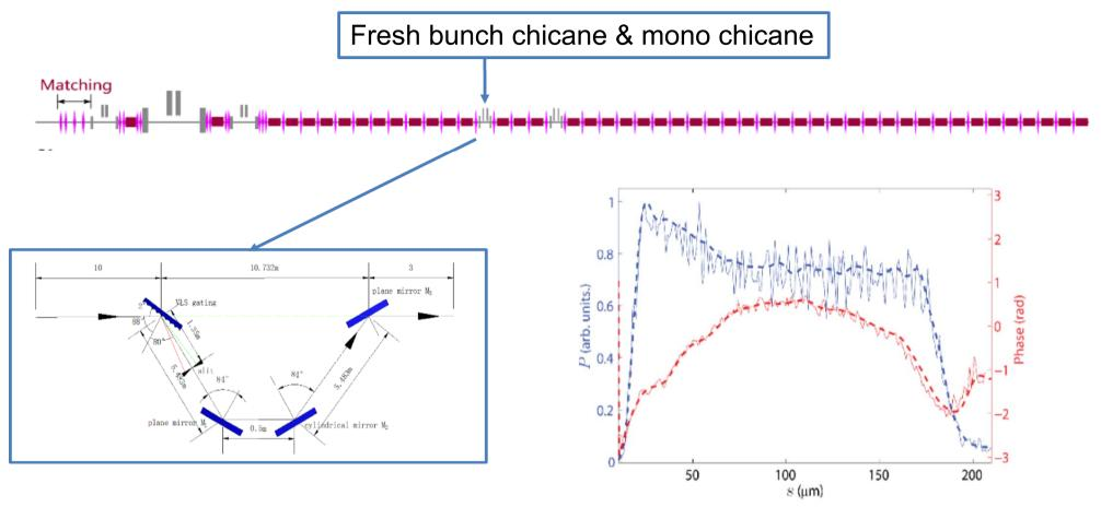
Longitudinal profile (blue) and phase (red) of the radiation pulse before (soiled line) and after (dashed line) the monochromator.
