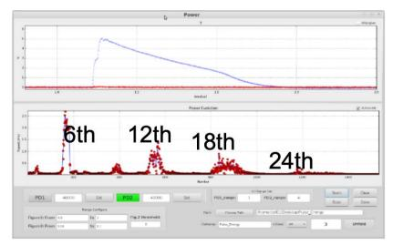
Scan the Gap of U40 and get coherent signal at various harmonics
