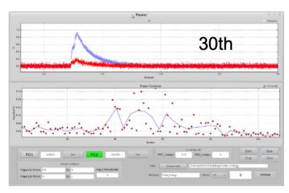
Scan the Gap of U235 and get coherent signal at 30<sup>th</sup> harmonic
