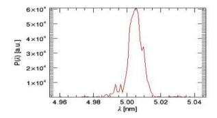
3.Radiation power and spectrum from the 2<sup>nd</sup> stage HGHG
