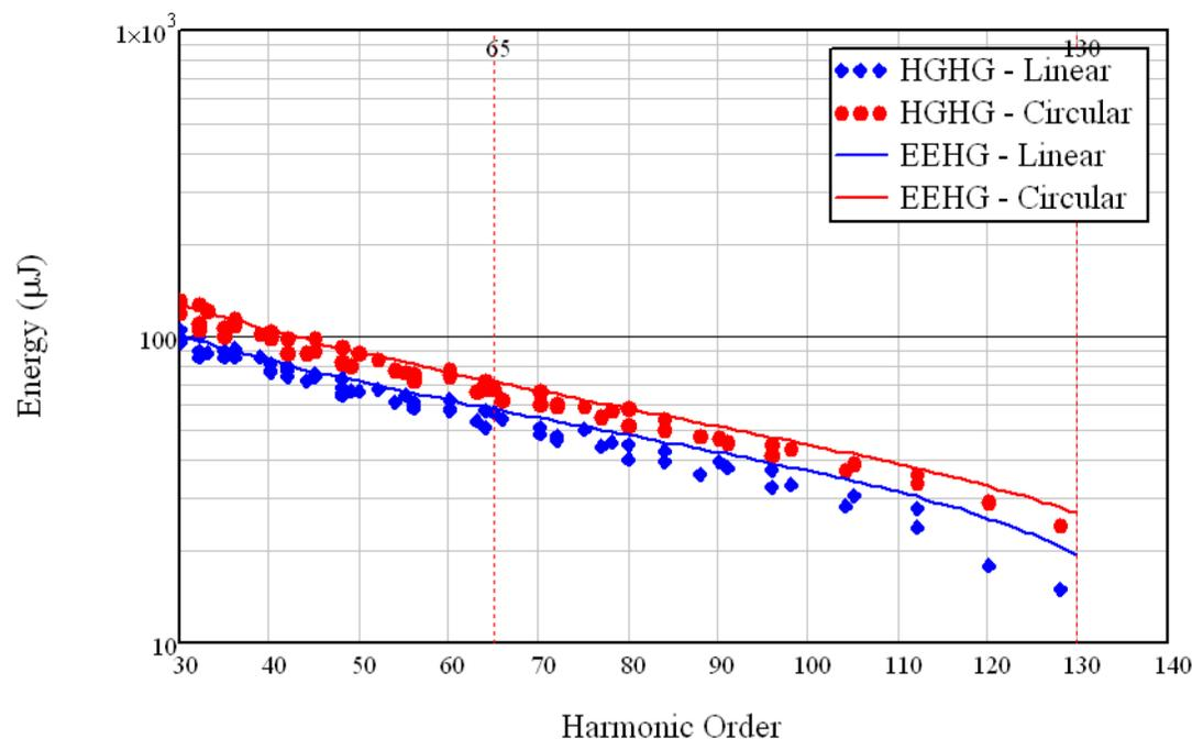
Both configurations, HGHG with fresh-bunch and EEHG provide similar performances, with a modest advantage of the latter.
