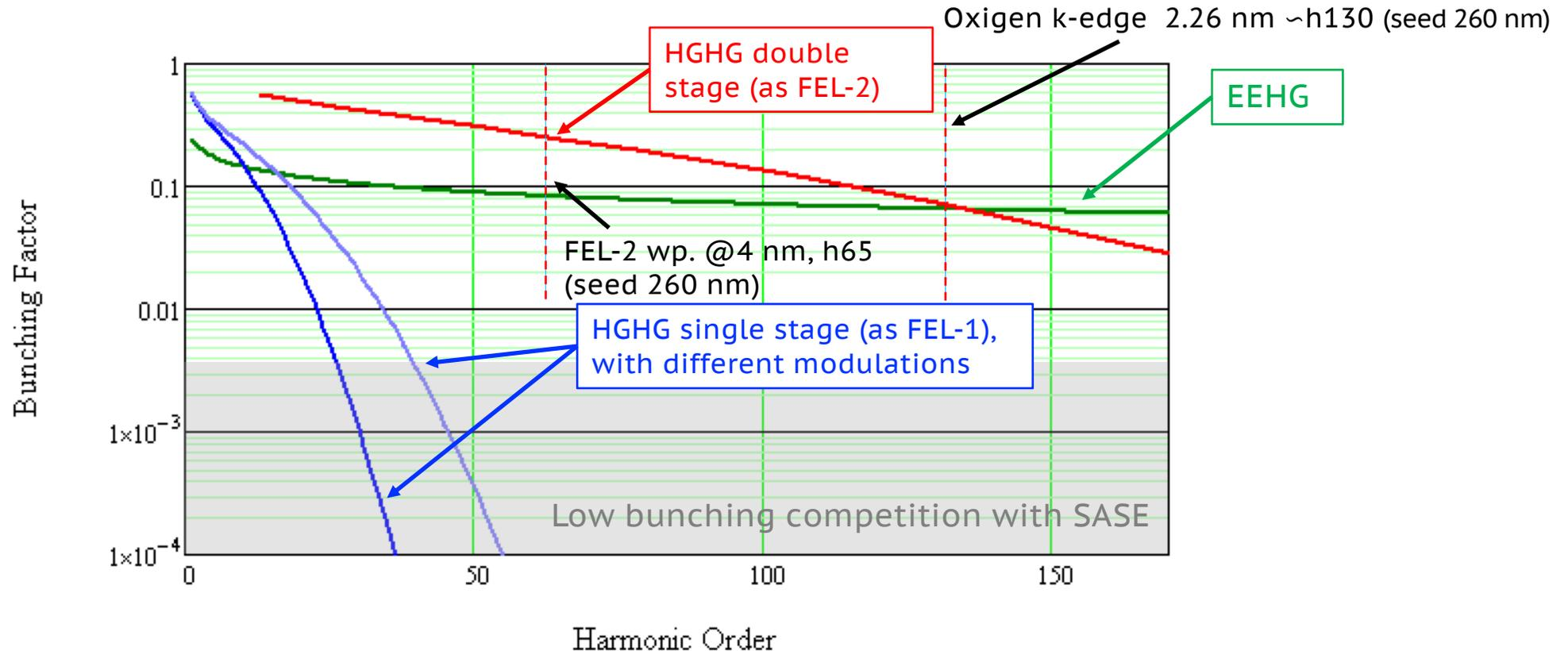
Both **EEHG** & **HGHG 2 stage with fresh bunch** are capable of generating bunching at harmonics as high as 130 (2 nm) **but we have to verify the impact of the degraded quality of the bunched beam on the FEL gain**
