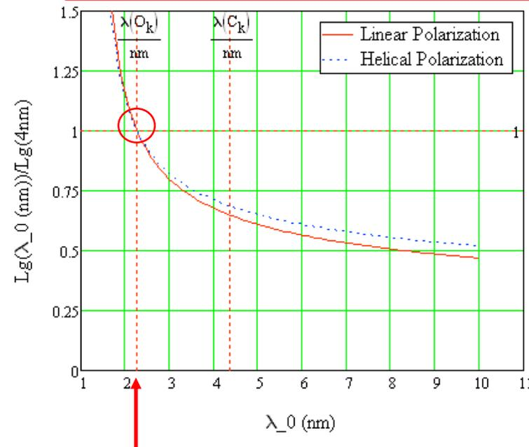
The linac upgrade together with a reduction of the undulator period from 3.5 cm to 3 cm provides at the Oxygen K-edge a **similar gain length to the one at 4 nm**
