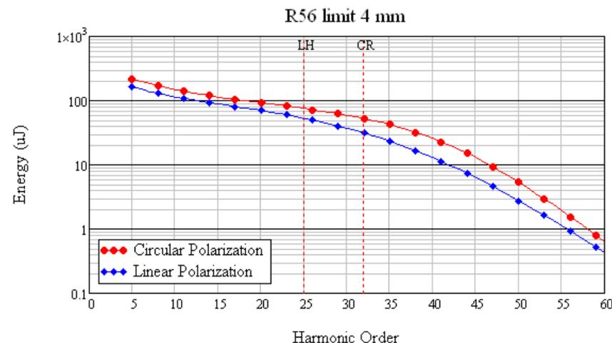
After the linac upgrade, assuming 1.8 GeV, 1 kA and a dispersion of 5 mm, the highest harmonics reaching saturation are **45 (5.5 nm)** and **34 (7.2 nm)** (**circular** and **linear**)
