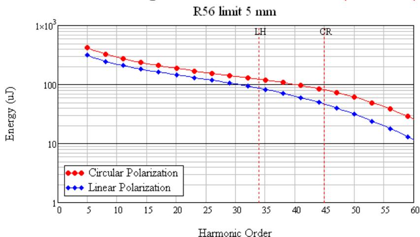
**These figures support the fact that FEL-1 is limited by the configuration (HGHG vs. EEHG) and can cover in EEHG the range 100 nm to sub-10 nm wavelengths**
