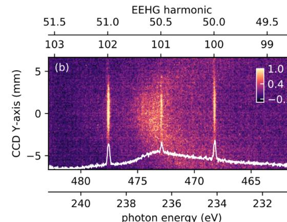
**FEL-2 EEHG H101** - Second order of diffraction and few seconds CCD integration time.
