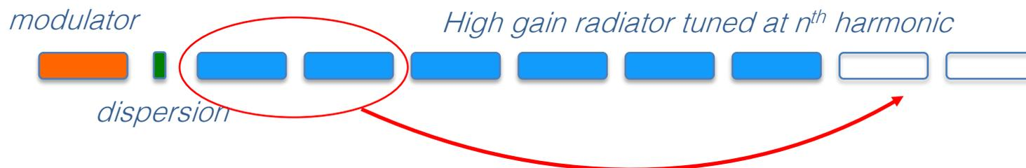
FEL-1 would require a first dispersion of about 5 mm, but **we have room for a dispersion up to 15 mm** which is of the order of what is required for FEL-2 optimised up to h130. **FEL-1 will be an ideal test bed for EEHG studies with large dispersion in the first chicane.**
