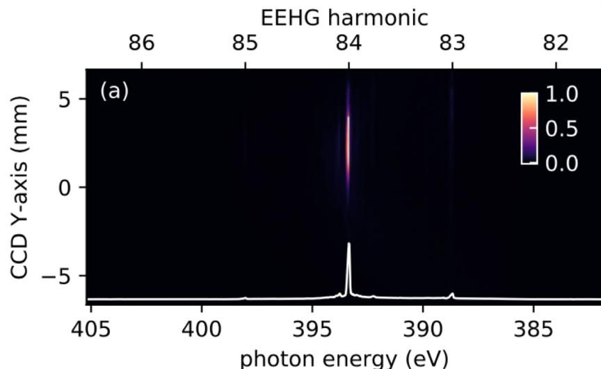
**Single shot spectra** with the EUV CCD (Andor) at 3 nm (shortest wavelength for first order of diffraction on PRESTO)
