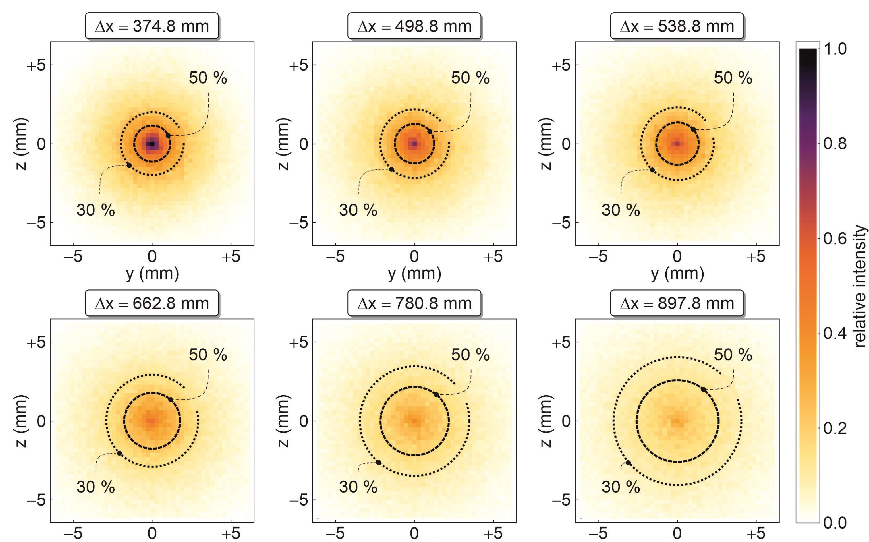
far field ( $\Delta x \geq 0.53 \text{ m}$ ) angular divergence:  $\Delta\beta_{\text{sim.}}^{(0)} = (7.0 \pm 0.1) \text{ mrad}$
