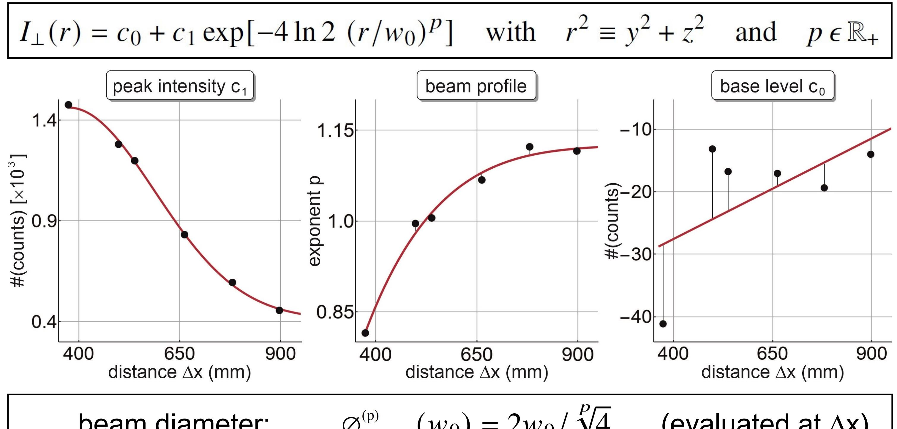
goodness of fit:  $\langle R^2 \rangle = (99.73 \pm 0.11) \%$  "coefficient of determination"
