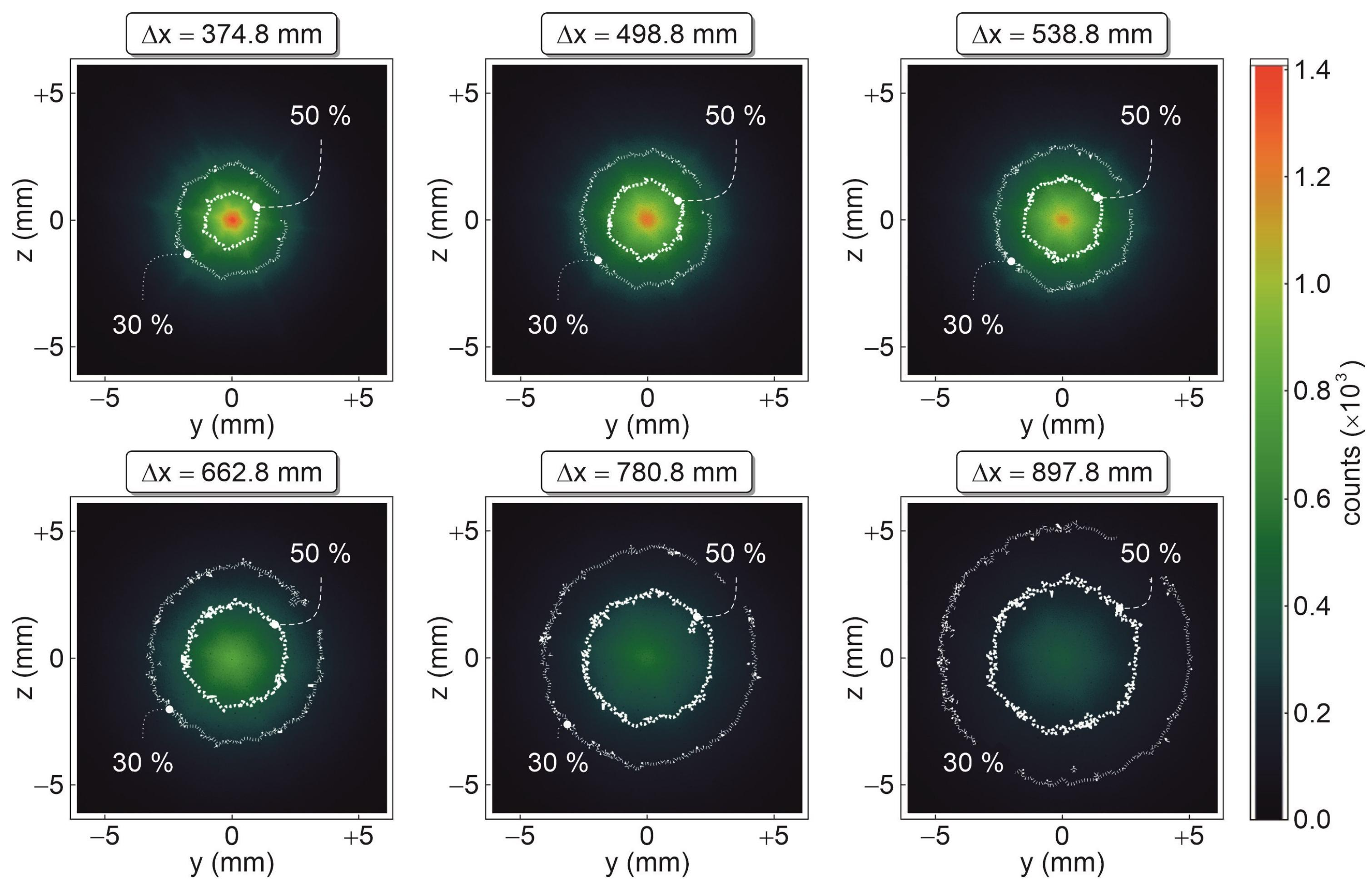
Nonlinear fit model to measured 2-D beam profiles  $I_\perp(r)$  and values
