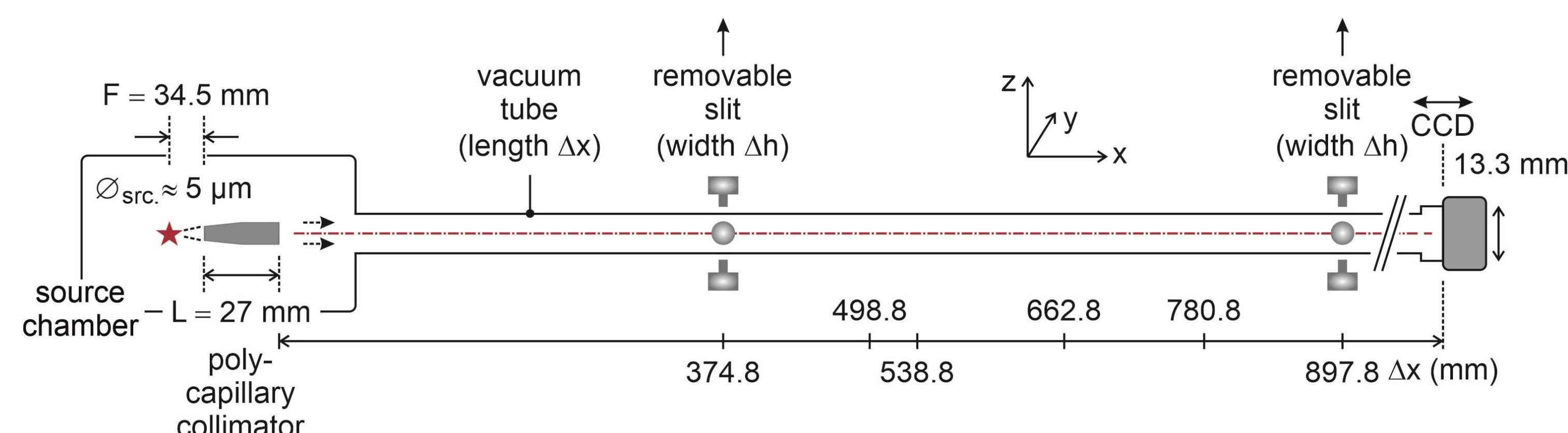
CCD at free-space distance  $\Delta x$  from exit aperture, or slit of width  $\Delta h$
