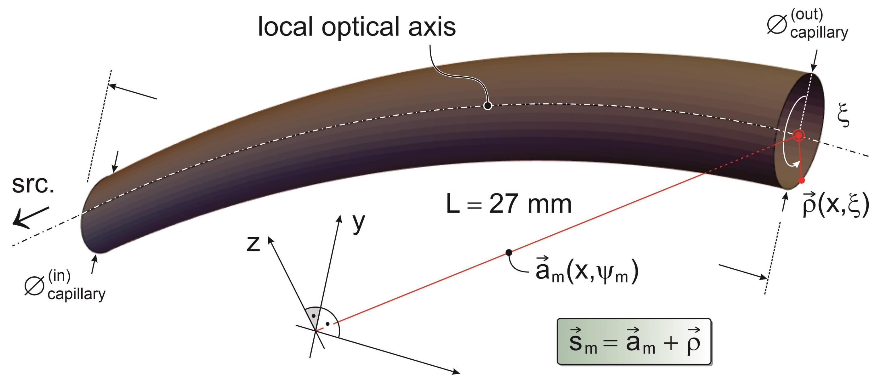
ellipsoidal curvature of local optical axis & tapered capillary diameter:
