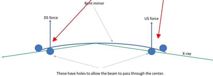
The 34-ID-C Nanofocusing KB-mirror is composed by two bendable mirrors, each equipped with 4 motors:
