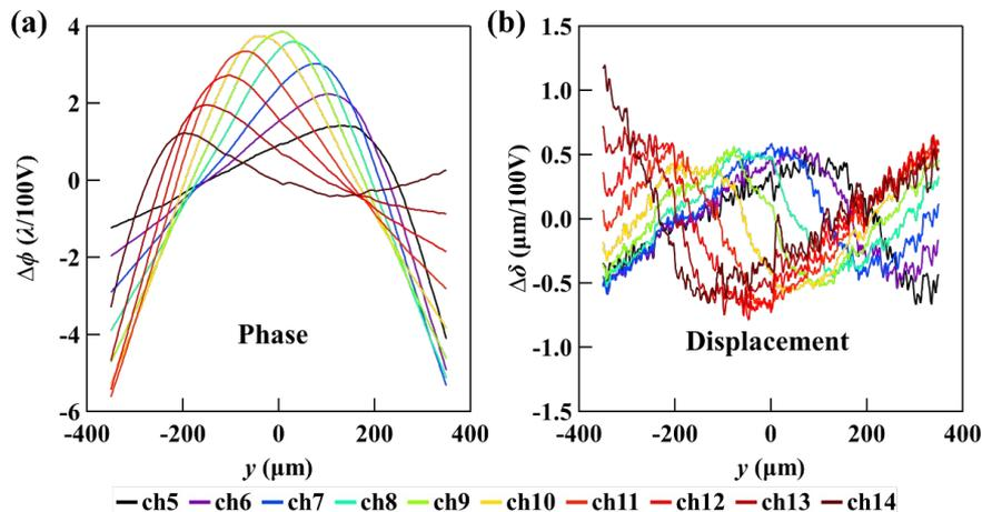
**Operating Conditions:** Measured response functions in terms of (a) wavefront phase and (b) speckle displacement changes per 100 V changes on each piezo electrode
