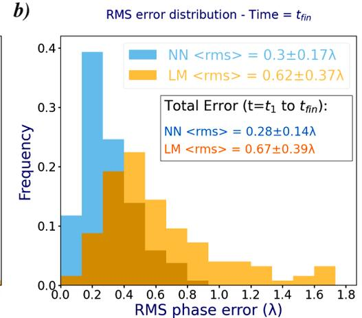
**Preliminary study:** mean RMS errors between the measured and prescribed shapes are 1.44 nm after one step and 1.51 nm after 10 steps (20 seconds). The predictive performance (figure error rms) of the neural network is  $\sim 2.5$  times better than the linear model across a full test dataset.
