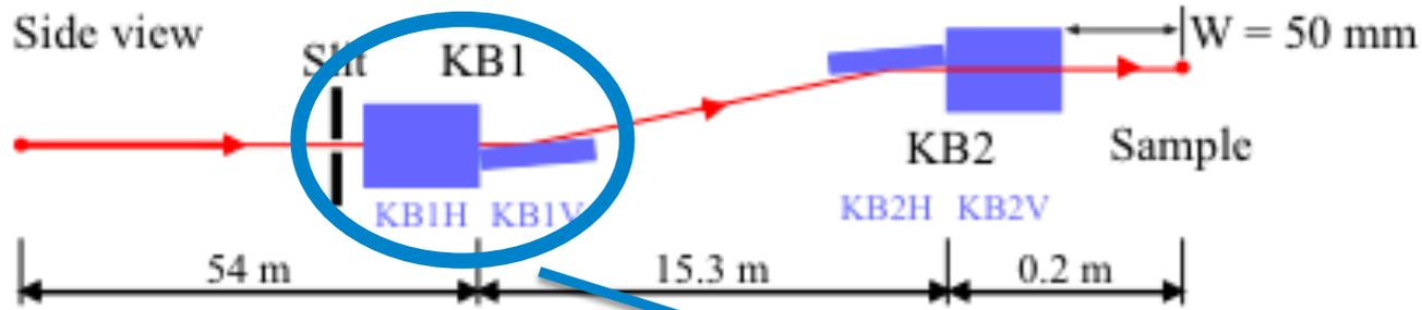
High-Quality bendable mirrors, using flexural nanopositioning stage system
