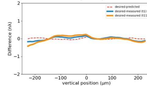
**Preliminary study:** Training and results in terms of **resulting surface shape** of the mirror vs applied voltages to the actuators
