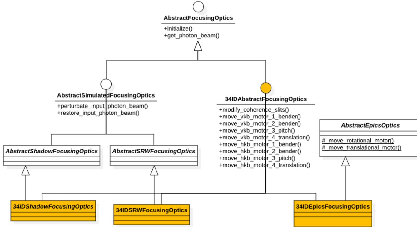
We developed an Object-Oriented framework to build the ultra-realistic simulation of the beamline, providing a software interface emulating the real controller of the beamline.
