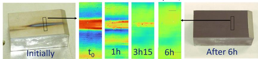
➤ Evaluate effect of extended ozone exposure upon optical micro-roughness of various coatings and Si substrates (spatial periods from 0.004 to 1.3 mm)
