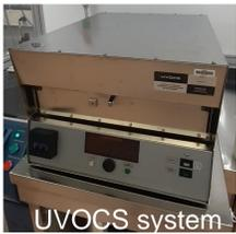
Low-pressure quartz Hg-vapour lamp, generates UV emissions in 254 and 185 nm range.
