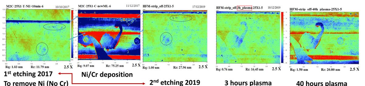
➤ New coating reveals residual surface deposits, that are transparent to micro-interferometer measurements.
