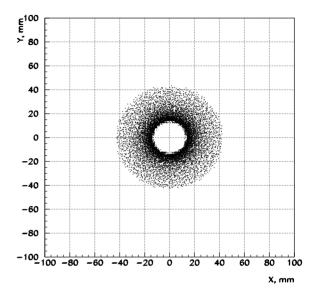
Figure 1: Transverse distribution of scattered electrons and positrons: ideal beam.
