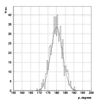
Figure 4: Azimuthal Bhabha scattered electron-positron distribution: for the positron beam angular dispersion  $\sigma_{\theta}=1.80\times 10^{-4} rad$
