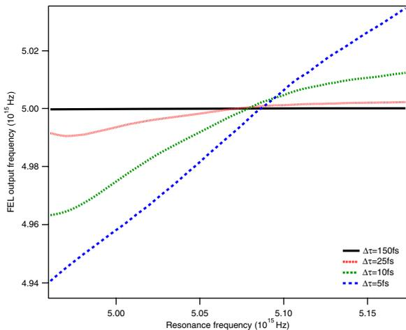
Fig. 4: (Colour on-line) FEL frequency *vs.* resonant frequency  $\nu_u$  (varied by changing the electron-beam energy), for different bandwidths (varied by changing the seed pulse duration,  $\Delta t$ ). The harmonic seed frequency is fixed at  $\nu_s = c/\lambda_s$  with  $\lambda_s = 60$  nm.
