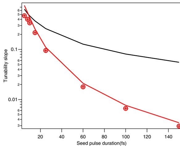
Fig. 5: (Colour on-line) Tunability slope as a function of the seed pulse duration: numerical results (crossed dots), data obtained from the standard frequency pulling equation (5) and from the modified equation (6).
