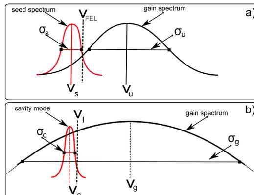
Fig. 2: (Colour on-line) a) Interplay between undulator (*i.e.*, gain) and seed spectra, leading to frequency pulling in a FEL. b) Interplay between active medium (*i.e.*, gain) and cavity mode spectra, leading to frequency pulling in a conventional laser. For symbols' explanation, see text.
