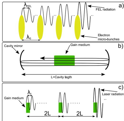
Fig. 1: (Colour on-line) Analogy between coherent FEL (a) and laser (b and c) emission processes. See text for an explanation of the symbols.
