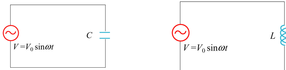
Figure 12.11.1 (a) A purely capacitive circuit, and (b) a purely inductive circuit.
