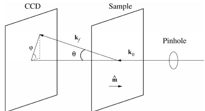
**Figure 2** Scattering geometry.
