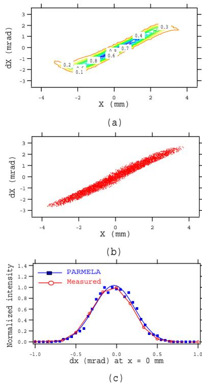
Figure 2: Phase space profiles of the electron bunch, (a) measured [3] and (b) calculated by "PARMELA". The measured and simulated divergences at the electron beam center ( $x = 0$  mm) is plotted in (c).
