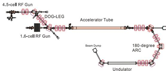
Fig. 1 Schematic view of the KU-FEL driver linac.
