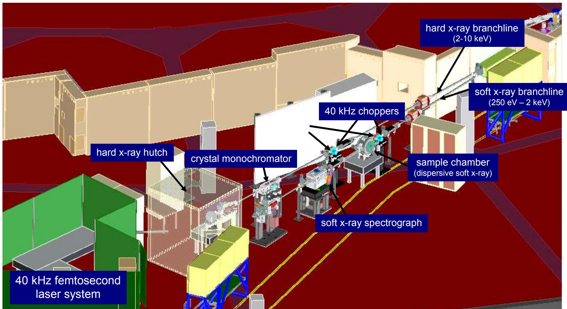
Separate beamlines for 100 fs time resolution studies using hard and soft x-rays
