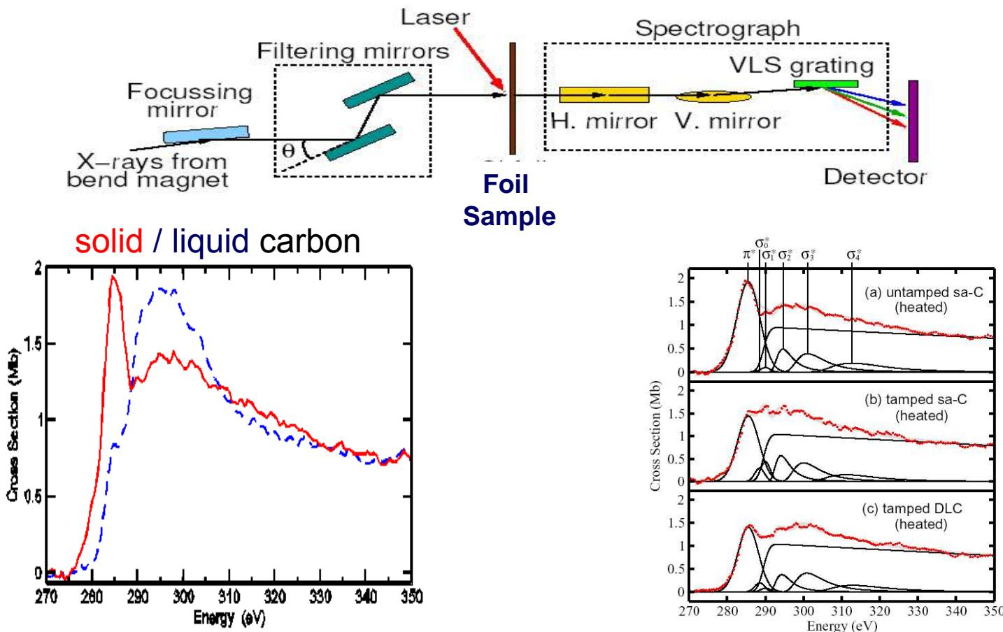
e.g., supports calculations indicating that the low-density phase of liquid carbon is predominately sp-bonded
