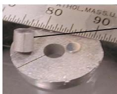
Shocked and incipiently fractured single crystal Al slug
