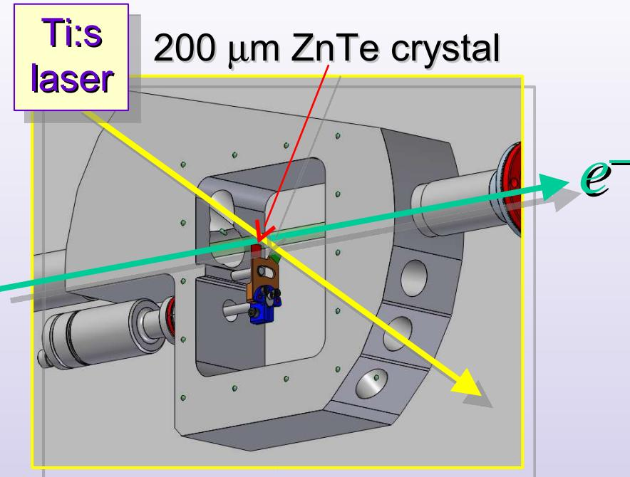
$e^-$  temporal information is encoded on transverse profile of laser beam
