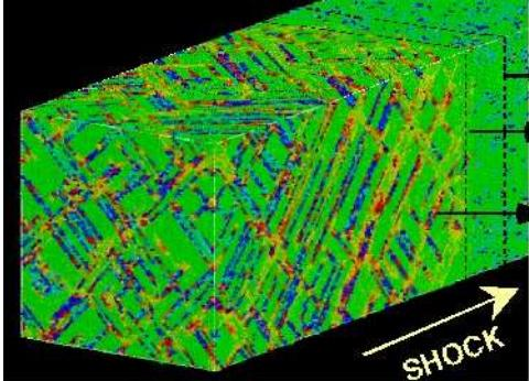
The figure shows a 3D visualization of a molecular dynamics simulation of FCC Cu. A shock wave is moving through the material, indicated by a diagonal arrow labeled "SHOCK". The simulation highlights several features: an "Elastic front" where the material is still elastic, a "Plastic front" where it begins to deform plastically, and a "Stacking Fault Network" where the crystal lattice structure changes. The background is black, and the simulation results are color-coded.
