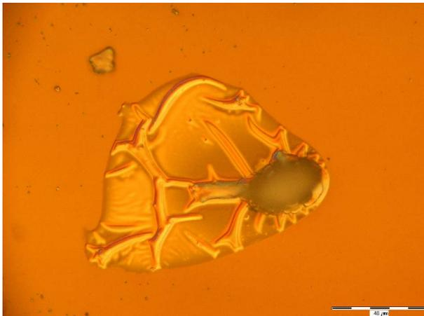
*Ablation of carbon coating on Si*
