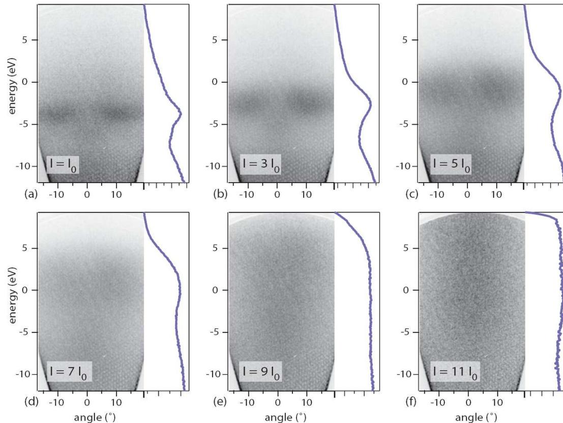
Figure 2: Angle resolved and angle integrated (solid lines) photoelectron spectra of the TiTe<sub>2</sub> valence band, taken at  $h\nu = 38.5$  eV and sorted according to increasing FEL-intensity from (a) to (f). Photoemission intensity is represented in a linear gray scale with dark corresponding to high intensity.
