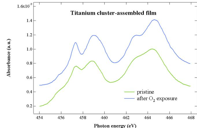
NEXAFS spectra at the L edge of titanium clusters of 350-400 atoms. Left: free clusters, 10 min/pt. Right: cluster assembled film.
