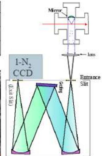
Visible fluorescence apparatus at Gas Phase.
