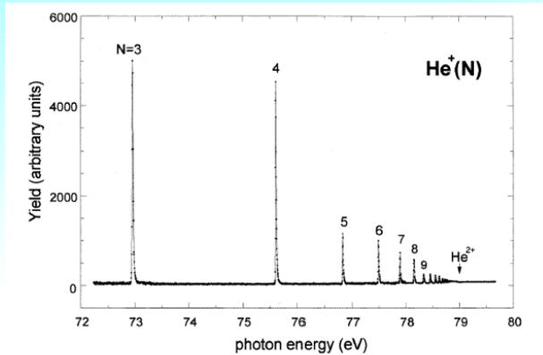
Figure 3. He<sup>+</sup> TPE spectrum covering the energy region from the  $N = 3$  ion state threshold through the He<sup>2+</sup> threshold. The dwell time is 6 s per point.
