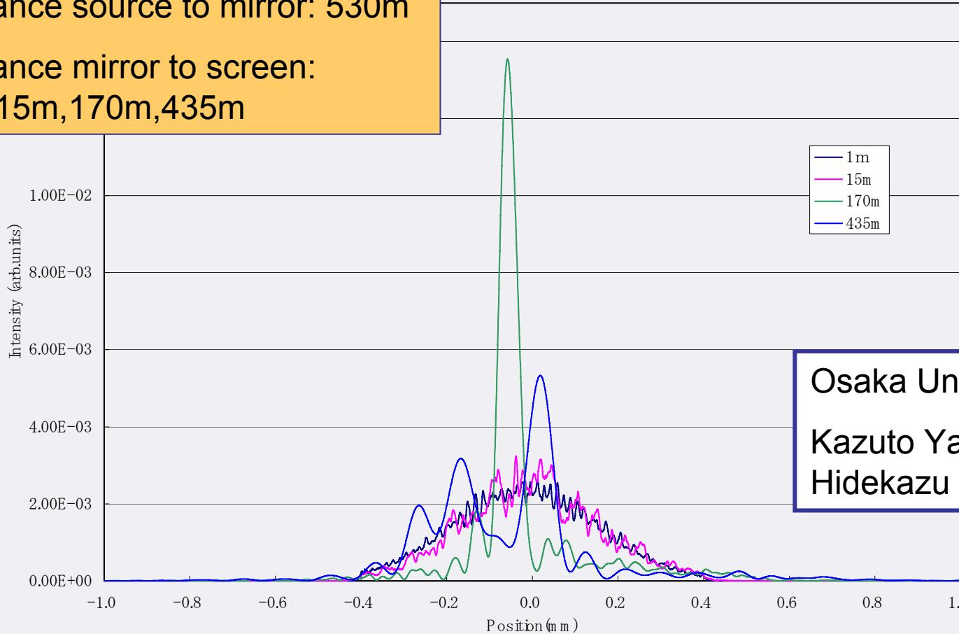
wavelength: 0.1nm, source size: 70micron, incident angle: 1.8mrad,
