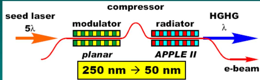
Cascade to HGHG FELs (to further enhance modulation and emit at higher harmonics) – progressively smaller slices of beam are selected
