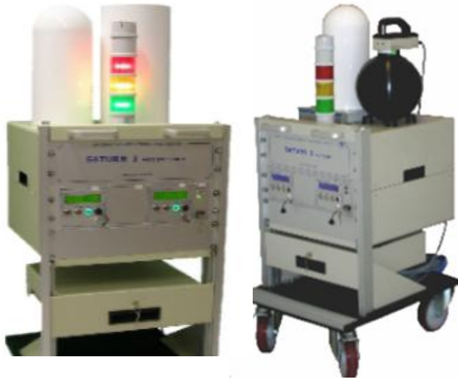
SATURN I Gamma/Neutron Monitors with fixed or removable probes
