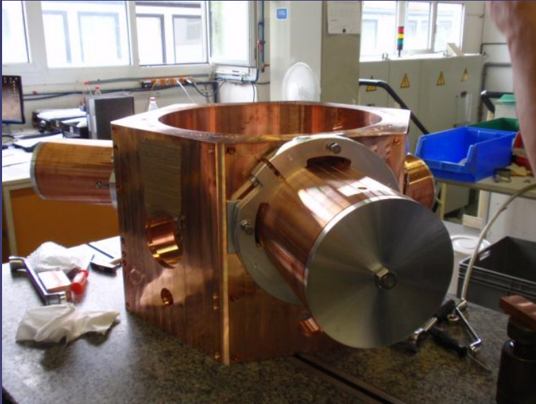
Cavity before e-beam welding
