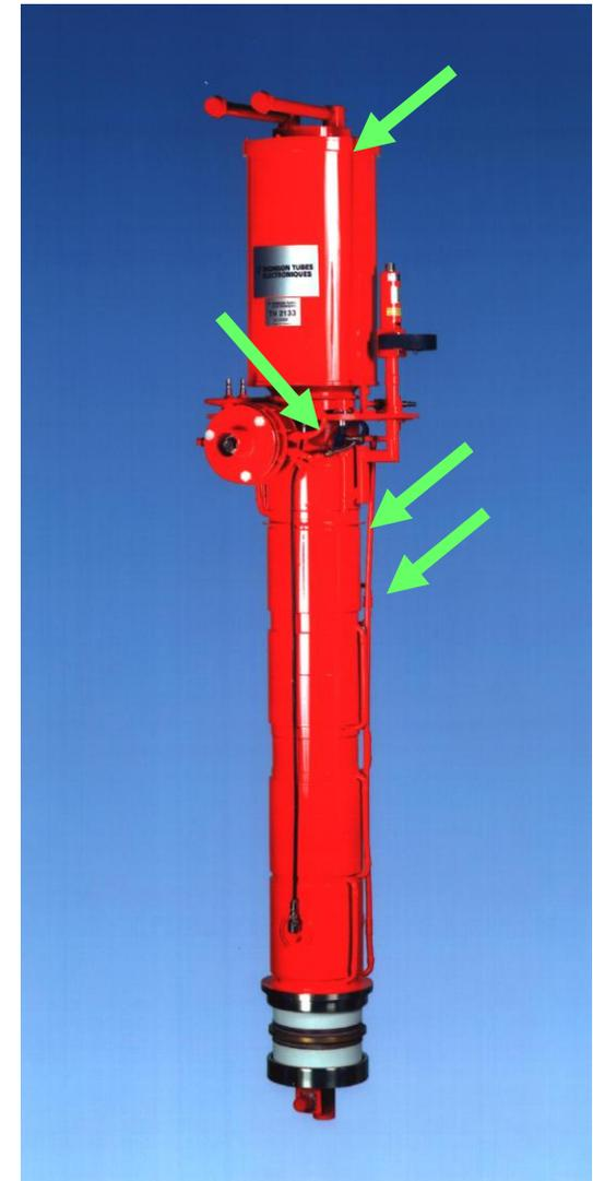
water leaks on new Thales klystron
