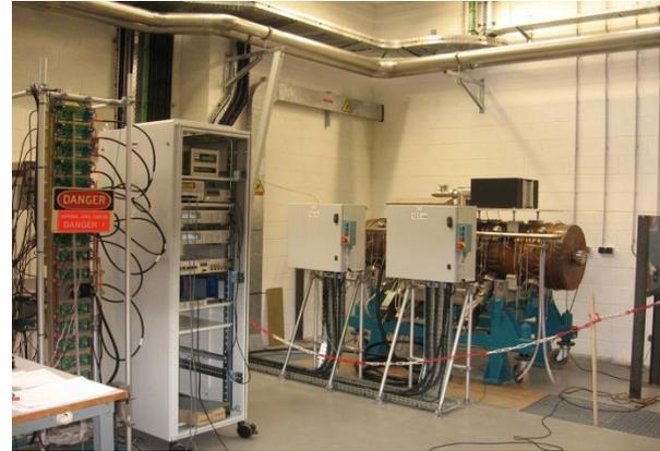
**Area test with high power voltage, water and spare BOOSTER Cavity**
