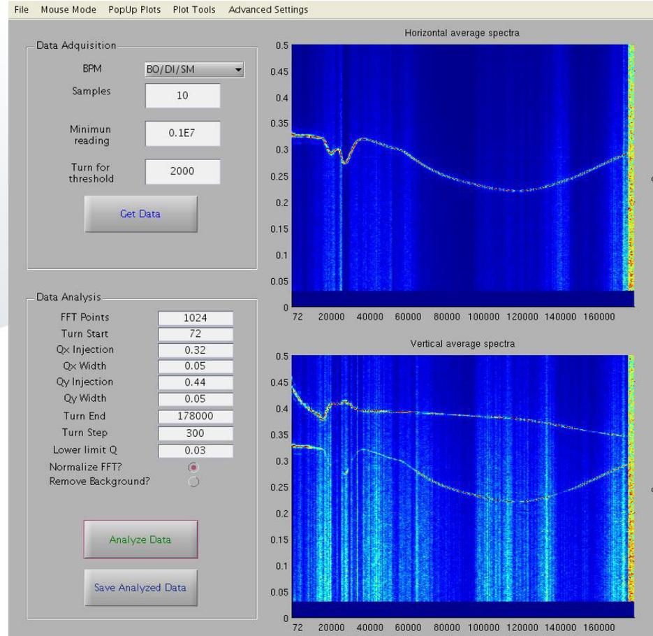
**Amplitude of beam kick increases in synchronism with beam energy, so to have enough power to excite beam w.o. killing it.**
