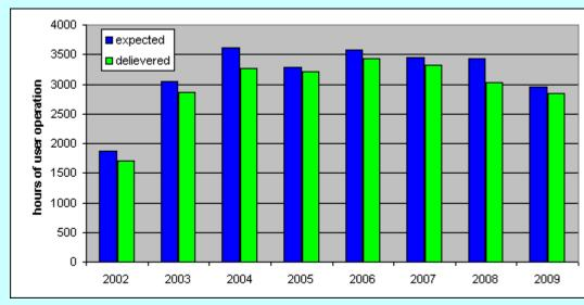
2008: Less availability due to e-gun vacuum leaks and longer start-up time (SULwiggler-AL-vac.-chamber)
