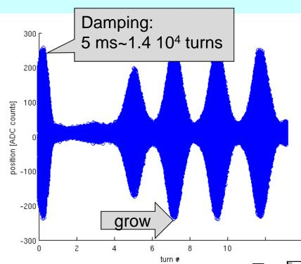
Feedback works at 2.5 GeV (user operation) Problems at 0.5 GeV (Injection): Phase RF Front-End Long. Instabilities always present
