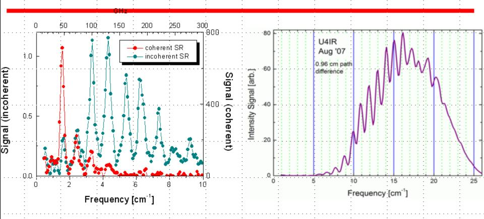
Interference model for line structure in both ISR and CSR pattern with  $\Delta f \sim 1 \text{cm}^{-1}$  spacing in two similar beamlines with different spectra ranges
