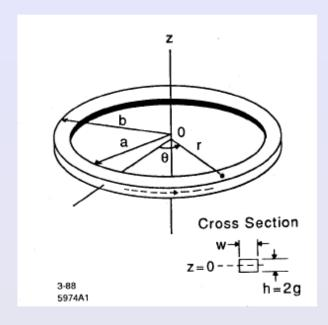
Solve for longitudinal electric field  $E_{\theta}(r, \theta, z, t)$  produced by the beam at the position of beam (r = R, z = 0), the Wake Field, which determines the dynamics of the bunch. The work done by the wake field per unit time is the negative of the Radiated Power.
