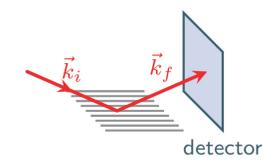
SAXS setup of HZB-BESSY. The in-vacuum Pilatus 1M detector allows for measurements at photon energies down to 1.75 keV.
