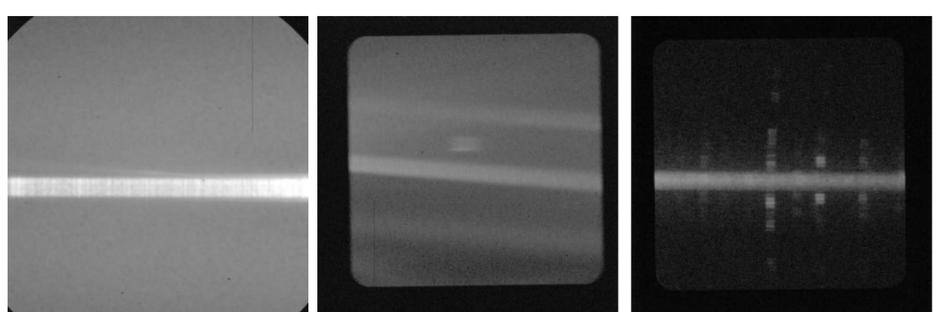
Representative diffuse scatter distributions between 0. and 1. order for the blazed, holographic and e-beam grating, from left to right. The grey scale is logarithmic and the same for all three pictures (1 to 5000).
