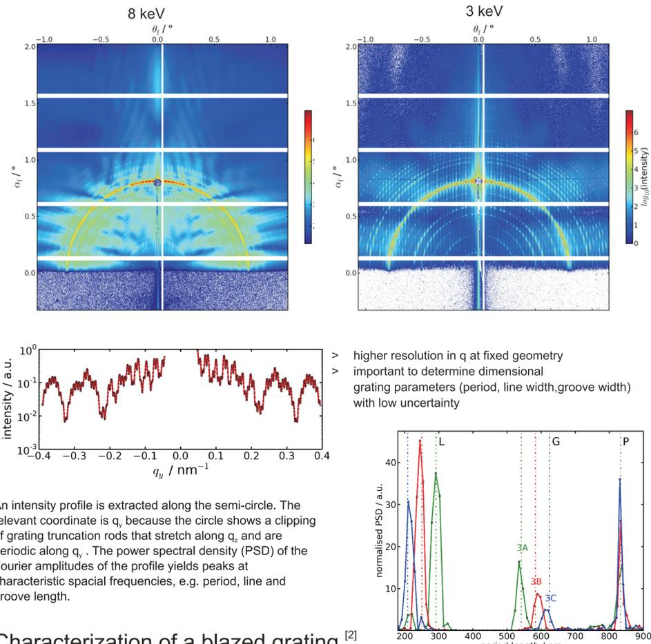
An intensity profile is extracted along the semi-circle. The relevant coordinate is  $q_y$ , because the circle shows a clipping of grating truncation rods that stretch along  $q_x$  and are periodic along  $q_y$ . The power spectral density (PSD) of the Fourier amplitudes of the profile yields peaks at characteristic spatial frequencies, e.g. period, line and groove length.
