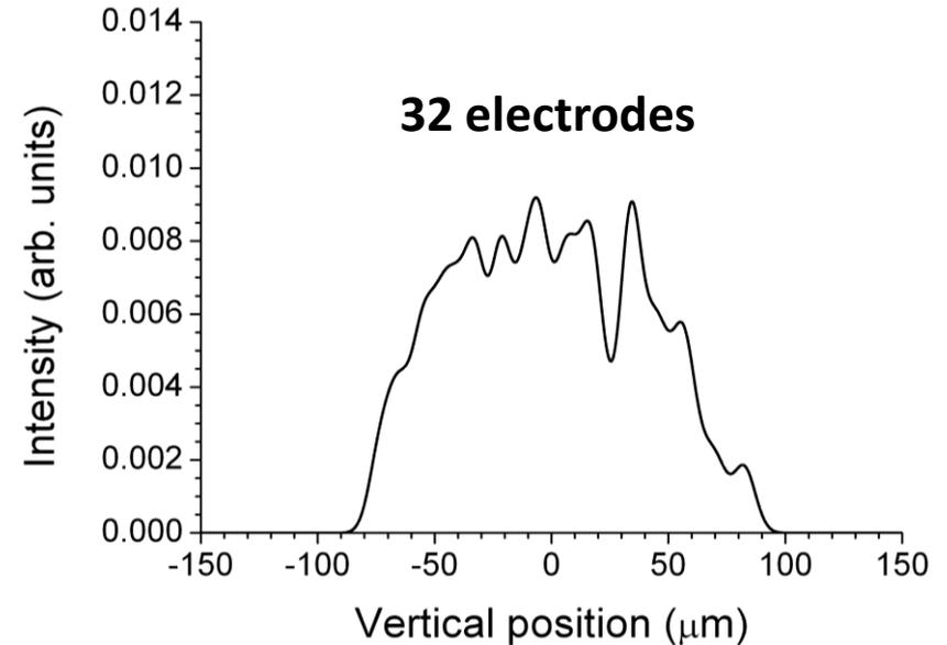
Convex additional curvature, requested beam size = 162.8  $\mu\text{m}$
