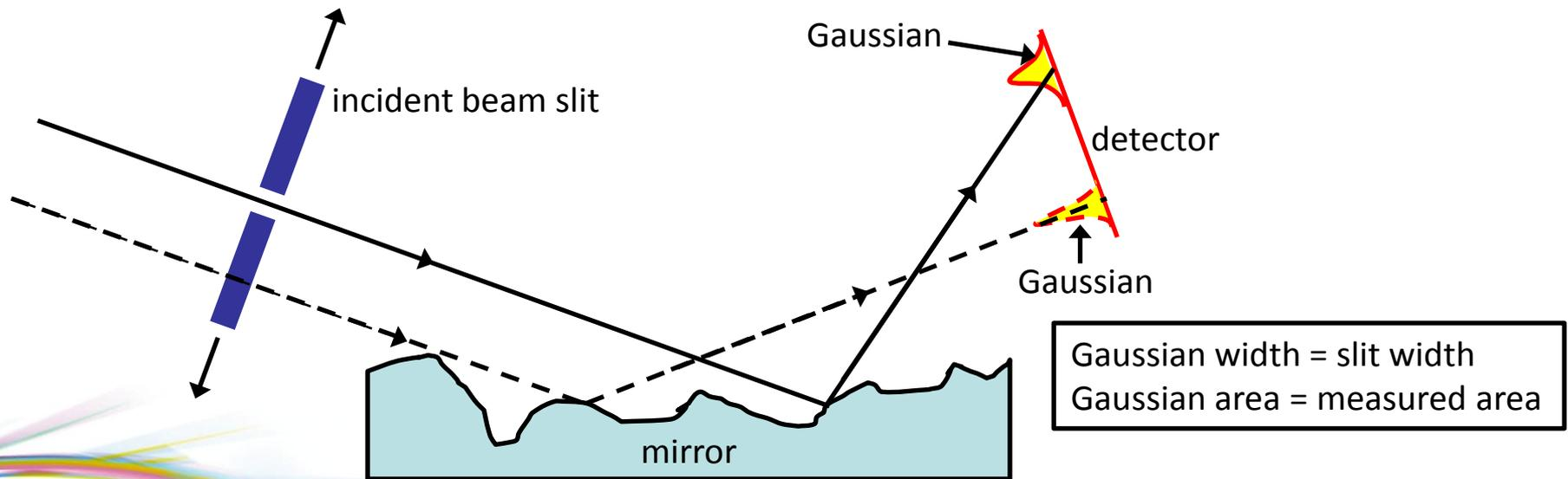
Each slit position produces a Gaussian on the detector.
