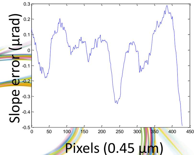
Minimum rms slope error =  $0.1457 \mu\text{rad}$
