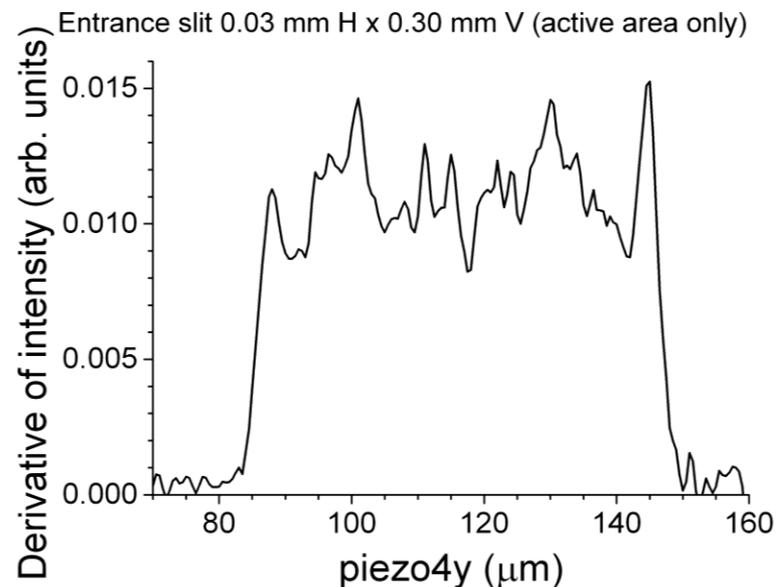
Defocused beam structure is not severe but still present.
