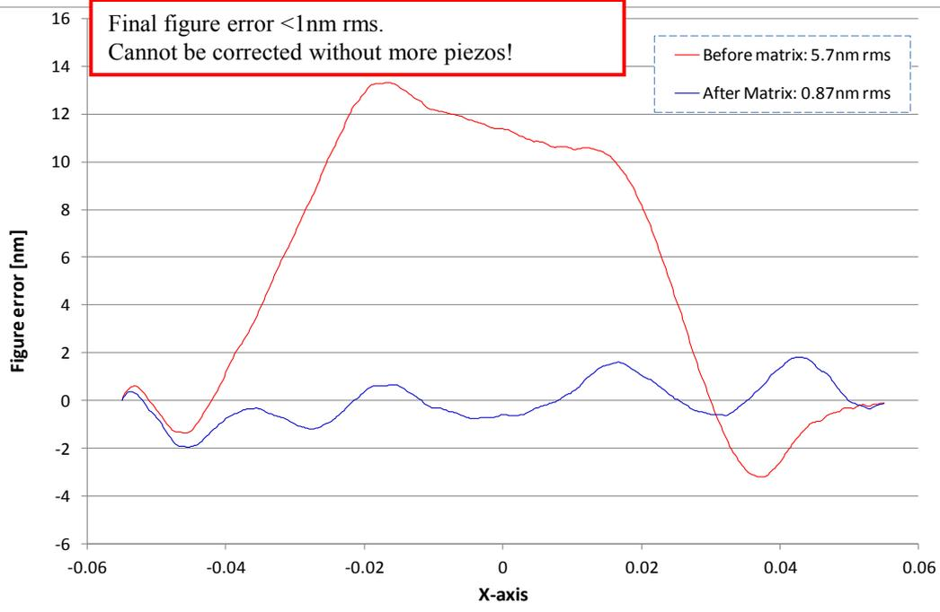
**Measured figure error of super-polished bimorph mirror on Diamond-NOM**
