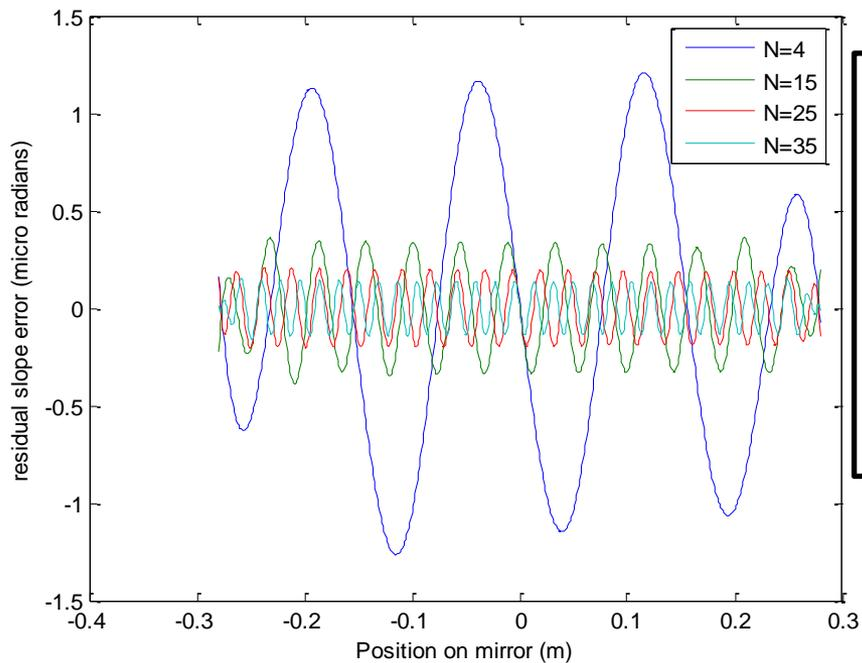
**Simulated bending of bimorph with  $N$  electrodes:**
