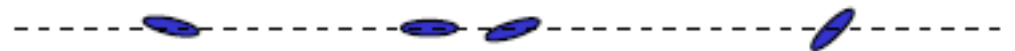
Figure 5: An asymmetric beam size scan with RF voltage indicates an incoming transverse-longitudinal correlation in the bunch, shown in the lower illustration, which is cancelled by the cavity at V(\sigma_{y\min}^2) .
