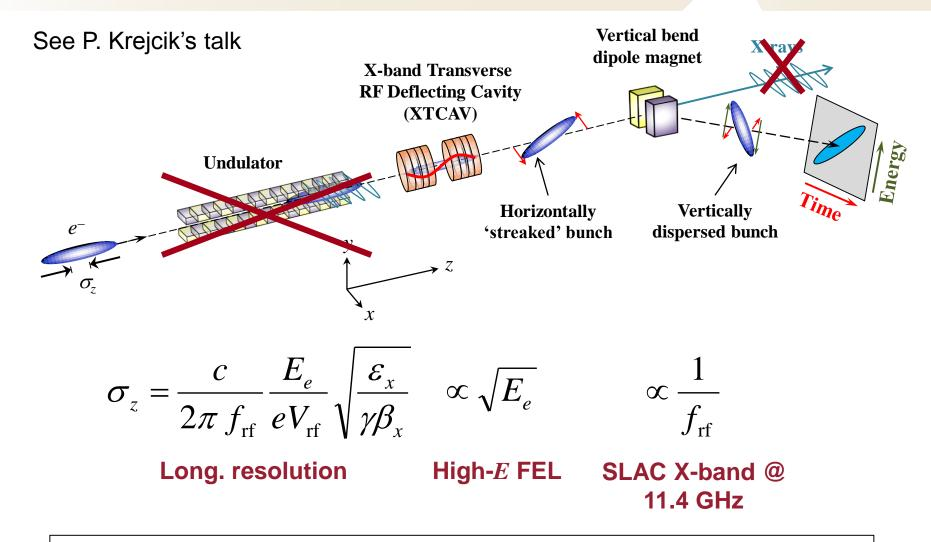
**Result:** < 1 µm rms @ 4 GeV, can now directly investigate final MBI impact
