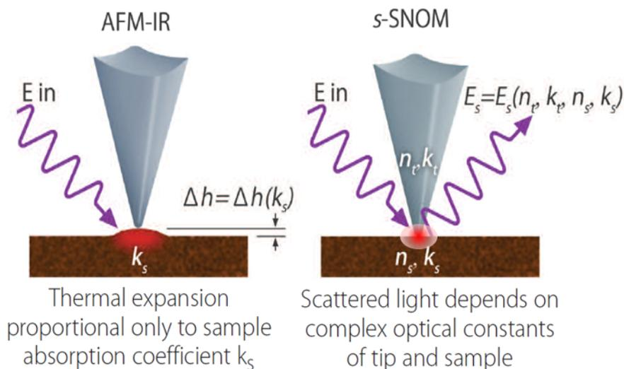
Figure: Close-up view of the laser light/AFM tip/sample interaction for the AFM-IR (left) and s-SNOM (right) experiments.
