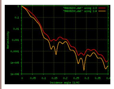
MAG\_sl example: difference between reflectivity of circular-plus and circular-minus polarized X-rays at E=849eV from 47A capped Ni film.
