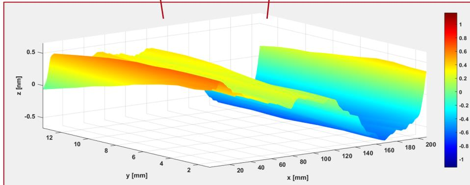
Measured error map, PV ~ 1.2 nm
