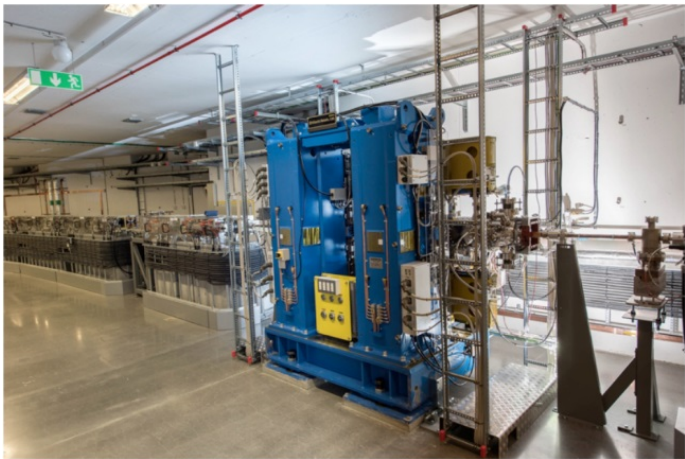
Biomax in-vac undulator 18 mm period 2 m length 4.2 mm min gap
