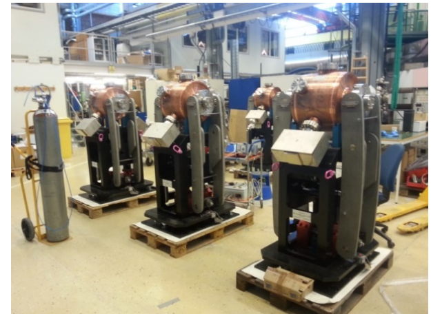
Passive 3 rd Harmonic Cavities
