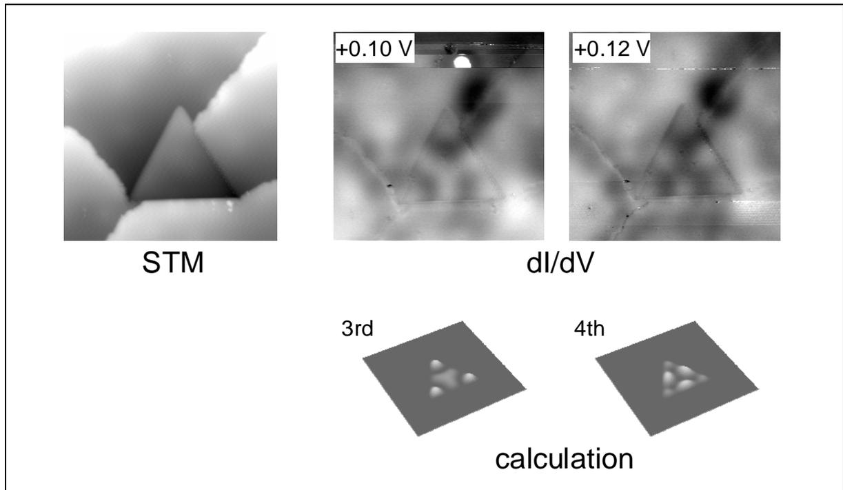
Figure 1: The STM image shows a triangular nanostructure (faultily stacked InAs crystal) at the InAs(111)A surface. The  $dI/dV$  images show the bias-dependent LDOS distribution within the nanostructure at 5.3 K. Image size is 67 nm x 67 nm. The  $dI/dV$  images correspond to calculated zero-dimensional states of the third discrete and fourth degenerate energy levels respectively. The bias difference of 20 mV is comparable with the energy separation between these energy levels.
