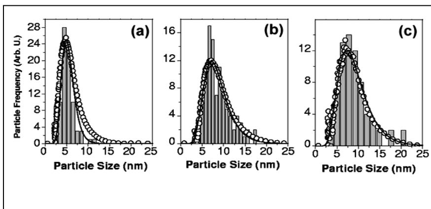
Figure 1: Particle size distributions for the sample S<sub>1</sub> (a), S<sub>1</sub> annealed 1 h at 320 °C (b), S<sub>1</sub> annealed 1h at 450 °C (c), bars - HRTEM results, circles - LFRS results, line - fit of log-normal distribution on the HRTEM distribution.
