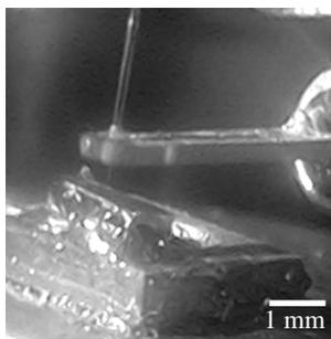
Fig.1 Picture of the low-temperature SNOM sensor. The optical fiber is mounted perpendicular to the quartz fork.
