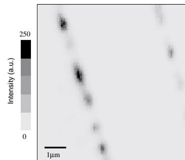
Fig.2 Intensity map of quantum wire PL emission.
