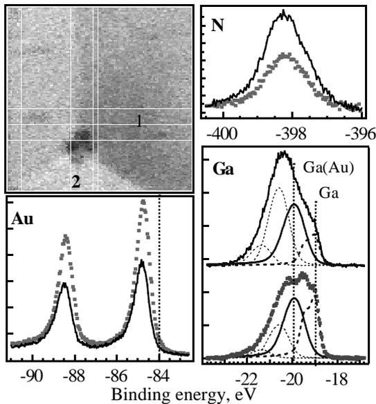
Fig.1. 22  $\mu\text{m}$  image of Au  $4f_{5/2}$  photoemission line with sets of spectra taken at points 1 and 2 which reveals different concentration of  $\text{AuGa}_2$  on different grains after annealing above  $750^\circ\text{C}$  but the same barrier height on different features.
