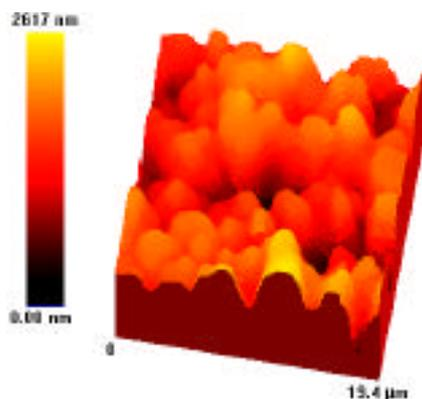
Figure 1. Layer of silicon compounds deposited on copper surface
