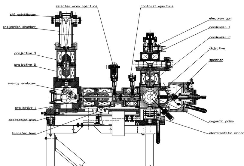
Fig. 1 Cross section of XPLEEM with the energy analyzer.
