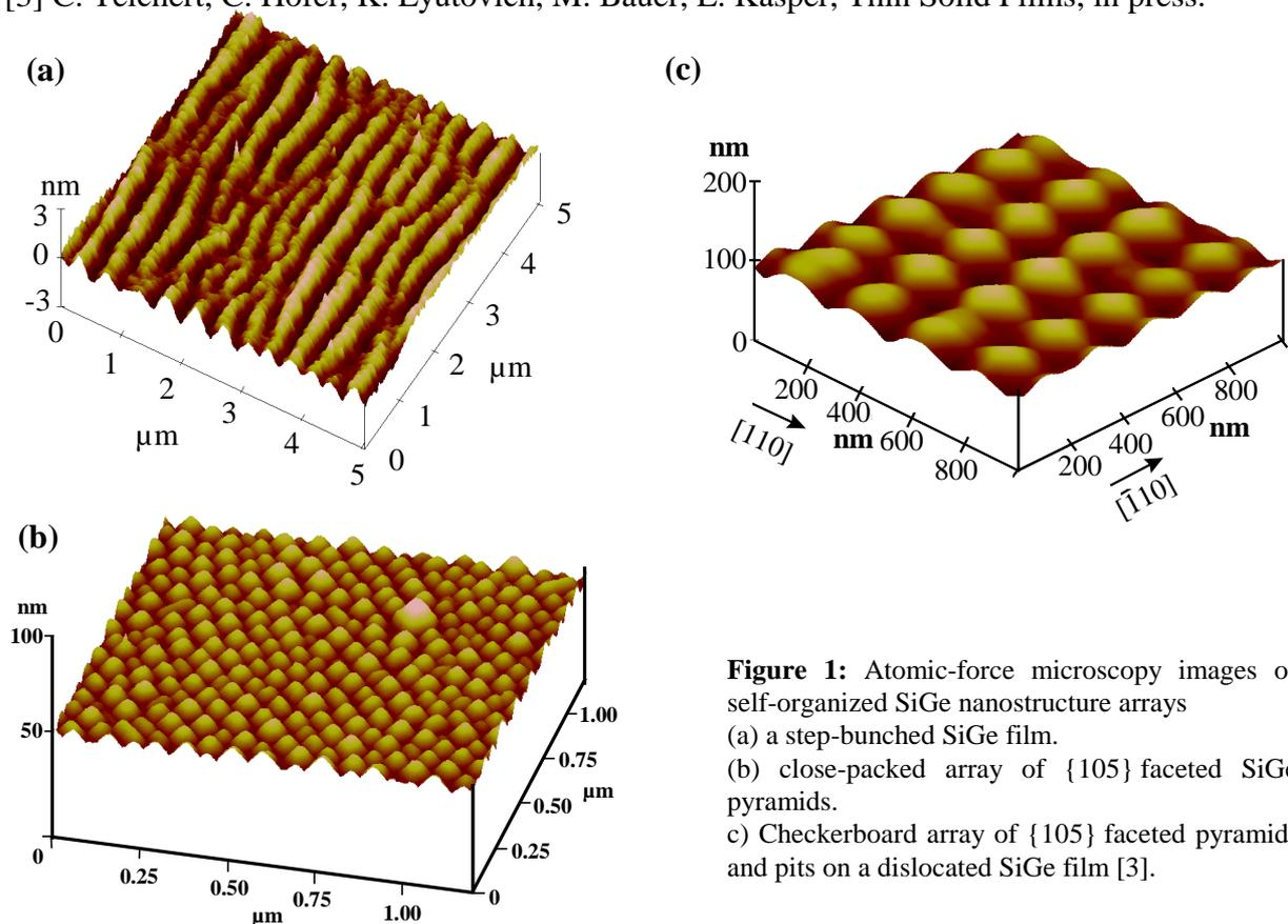
**Figure 1:** Atomic-force microscopy images of self-organized SiGe nanostructure arrays
