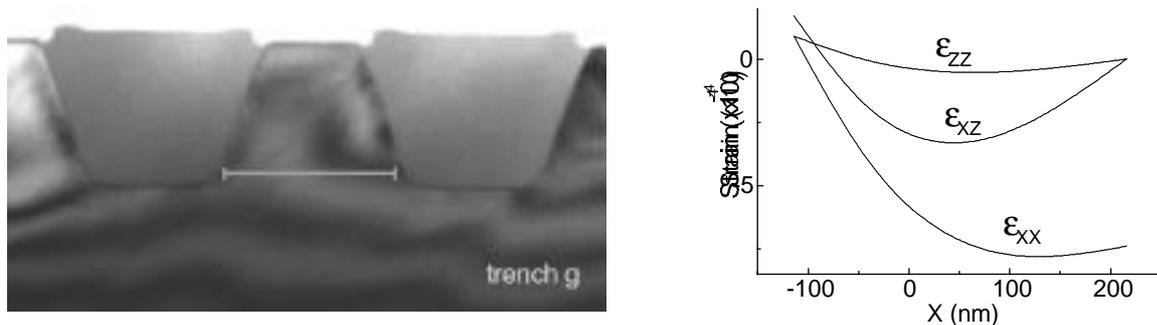
Figure 1. (left) TEM image of a 0.37  $\mu\text{m}$  large active area bounded by two STIs. The horizontal line represents the cutline along which the CBED patterns have been taken, giving rise to the strain field reported on the right.
