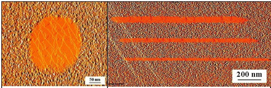
Figure 1: An open window and a line-and-space pattern. The minimum feature size attained is 25nm and rms edge roughness of line patterns is less than 3.5nm.
