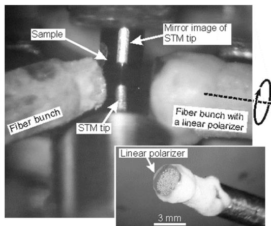
Figure 1: Photon detecting STM
