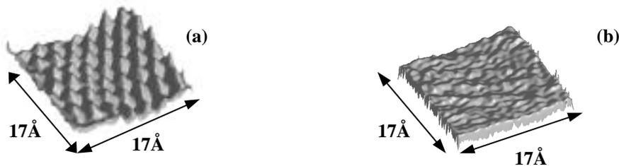
Fig. 1. *In-situ* STM images of (a) pristine HOPG and irradiated with 200 MeV Au<sup>8+</sup> ions at the fluence of  $2 \times 10^{13}$  ions cm<sup>-2</sup>.
