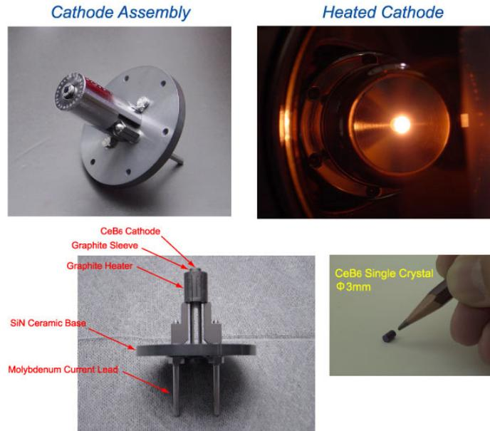
Fig. 2 : CeB<sub>6</sub> cathode assembly.
