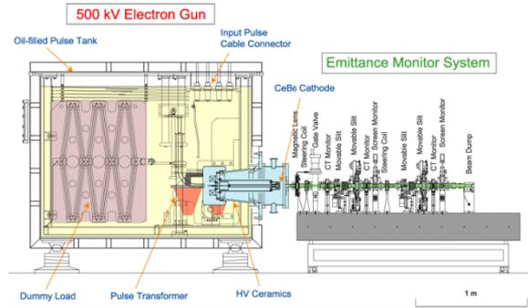
Fig. 1 : A side view of the CeB<sub>6</sub> electron gun with an emittance monitor bench.
