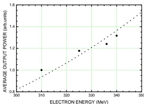
Fig.1. Dependence of average output power on the beam energy. Solid circles and solid curve indicate the observed power and an expected curve proportional to the 4<sup>th</sup> power of the beam energy.
