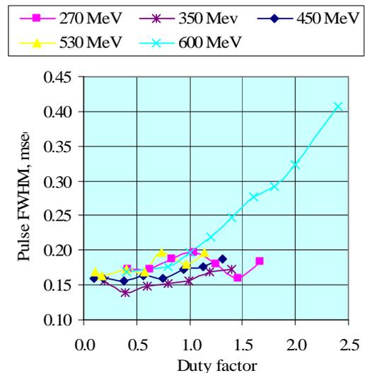
Figure 3. The dependence of the giant pulse width on the duty factor.
