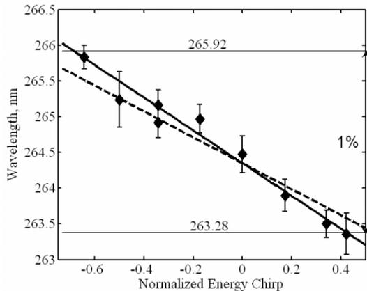
Fig. 4: Measured dependence of the HGHG central wavelength on the normalized energy chirp. Error bars represent measured single-shot HGHG linewidth. Tunability range of one percent lies between horizontal lines. First fit (dashed line) is calculated based on the DS calibration. Second fit (solid line) takes into account dispersion in the radiator.
