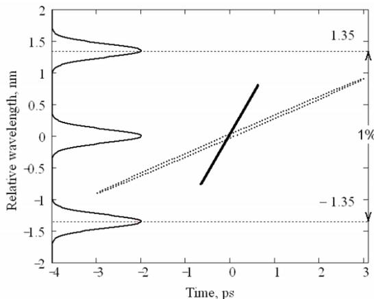
Fig. 5: Representation of the seed laser (dashed ellipse) and electron beam (solid) in wavelength (ordinate) – time (abscissa) coordinates. Tunability range of one percent lies between horizontal dotted lines. Measured tunability range exceeds the seed laser bandwidth.
