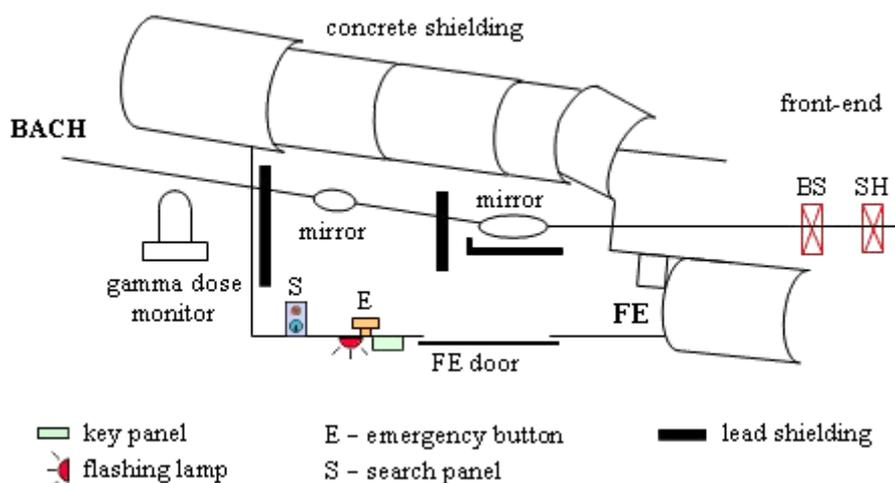
Figure 27. Scheme of the beamline.
