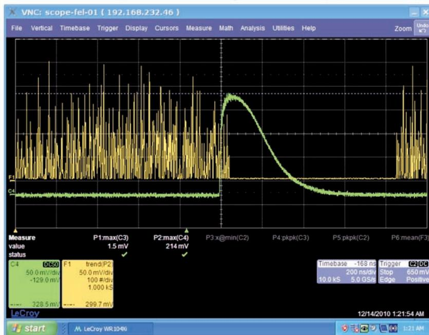
**Figure 1.** Seeded coherent emission from FEL-1 measured by means of a fast photodiode located in the FERMI experimental hall. The undulators were tuned at 43 nm. The green trace shows the time profile of a single pulse with the photodiode in saturation. The yellow trace shows a series of seeded FEL pulses being turned on (left) and off (center-right) by changing the superposition between seed laser pulses and electron pulses.
