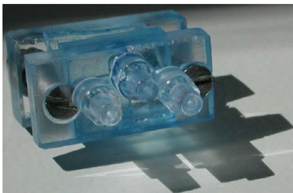
Figure 1. Mechanically fabricated mixer with cross channel. Triangle cross section 100 \mu\text{m} high, 200 \mu\text{m} wide.
