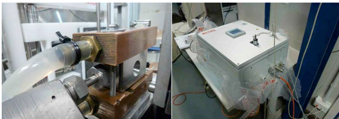
Figure 1. The installed high pressure cell with temperature control unit at the SAXS beamline (left) and the control unit of the high pressure generator in the control cabin (right)
