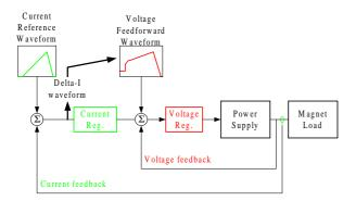
Figure 2: Ramping Power Supply Block Diagram
