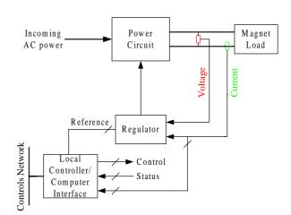
Figure 1: Generic Accelerator Magnet Power Supply
