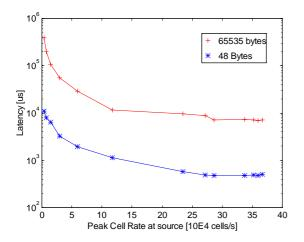
Figure 4: Communication latency as a function of the Peak Cell Rate at the source (AAL-5, 155 Mbit/s link)
