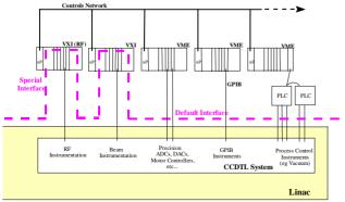
Figure 2 – Interface to SNS Control System
