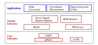
Figure 2: Vertical Dependencies: Module Layers.
